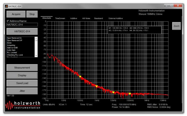
Figure 6 GUI screenshot showing the phase noise measurement of a 100MHz OCXO, down to a 1 Hz offset.
