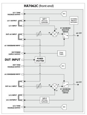
Figure 1 HA7062C front-end block diagram.
