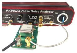
Figure 2 The external LO mode function was developed primarily for evaluating crystal
