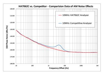
Figure 4 AM effects can add an uncharacteristic bump or null in the phase noise response.
