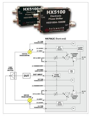
Figure 3 Adding a pair of electronic phase shifters enables the HA7062C to perform fully automated, cross-correlation, additive phase noise
